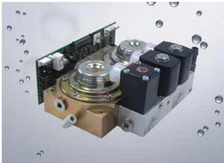
The older version of the insufflator block made of milled aluminium, partially equipped with specially manufactured valves
