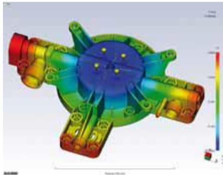
Results of the MoldFlow analysis with respect to the filling time of the injection mould during the production process for the new insufflator block made of polycarbonate (view from below)
