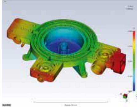
Results of the MoldFlow analysis with respect to the filling time of the injection mould during the production process for the new insufflator block made of polycarbonate (view from above)
